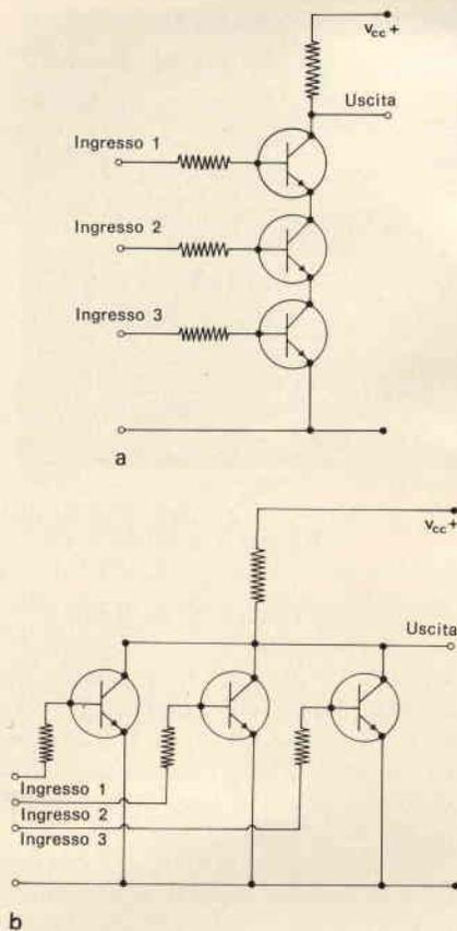
Fig. 2 - Circuito NAND in (a) e circuito NOR in (b).
